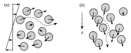
FIGURE 1. Schematic of particle velocities and the trajectory of a test particle in a suspension subject to (a) shear flow and (b) sedimentation.
