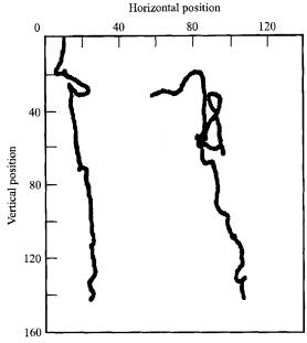
FIGURE 2. Trajectories of two test particles in the interior of a suspension subject to sedimentation; the positions are non-dimensionalized by the particle radius (adapted from Nicolai *et al.* 1995).
